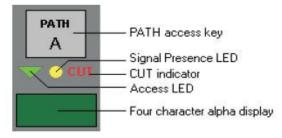
The console will enter Copy Mode. The alpha displays associated with the Path access keys will flash alternately between the path names and **COPY**.
