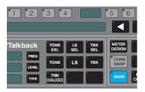
To select which **Bank** to use, press the **Bank** button in the **Quick keys** section of the console. Now use the numbered **1-6** buttons above to select the desired Bank.
