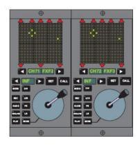
The twin Joystick module is used to pan up to two signals across surround speaker destinations.
