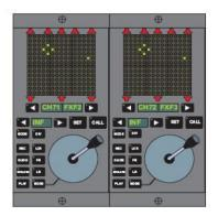
The twin joysticks allow fully automated surround panning of any two paths simultaneously. Any number of paths can be panned in turn using the joysticks with repeated passes.
