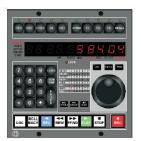
The MCS Panel is a hardware option that is used to control multiple transport devices (up to the first eight that are detected on power up).
