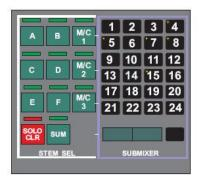
The led(s) for the currently selected Stem(s) in the **Stem Sel** section will flash.
