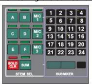
Press the **A** key in the **STEM SEL** section of the Surround Monitoring panel.
