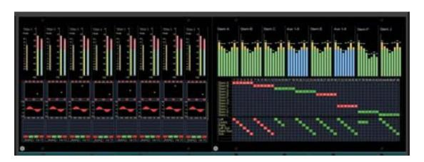
The DFC Gemini has 2 types of meter display, one for above the faders (above left), and a dedicated Centre meter panel (above right).
