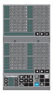
Lower Routing Section Routing mode is activated when a button is held down on the Upper Routing Section.
