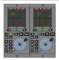
The Joystick Module has two **MODE** keys for selecting automation modes of the **Divergence** controls and the panning axes.
