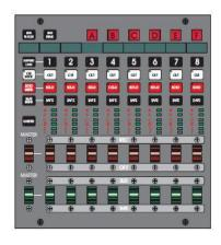
The PEC/Direct panel provides stem recorder control and configuration of the film stems.
