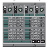
The meter selection controls are used to assign a port to each of the Wild meters in a Meter Design.
