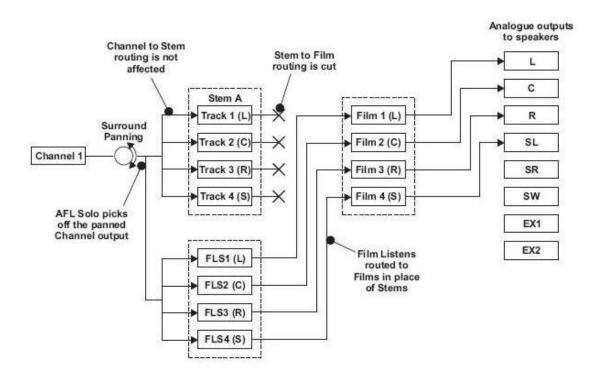
The panned signal from the selected path will now be routed to the Film Listen paths and then to the Film paths to output to the monitor speakers.
