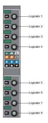
The function of the Logicators depends on the selection made with the Function Selection keys in the middle. By convention, the Logicators are referred to as Logicator 1 (top) to Logicator 8 (bottom).
