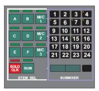
Press and hold the blank key next to the alpha display on the Submixer section.
