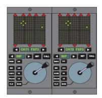
**The Joystick Module** provides an intuitive means of panning a signal in a surround sound field.
