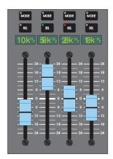
Press the fader **SEL** key for the required band (the integral led will illuminate orange).
